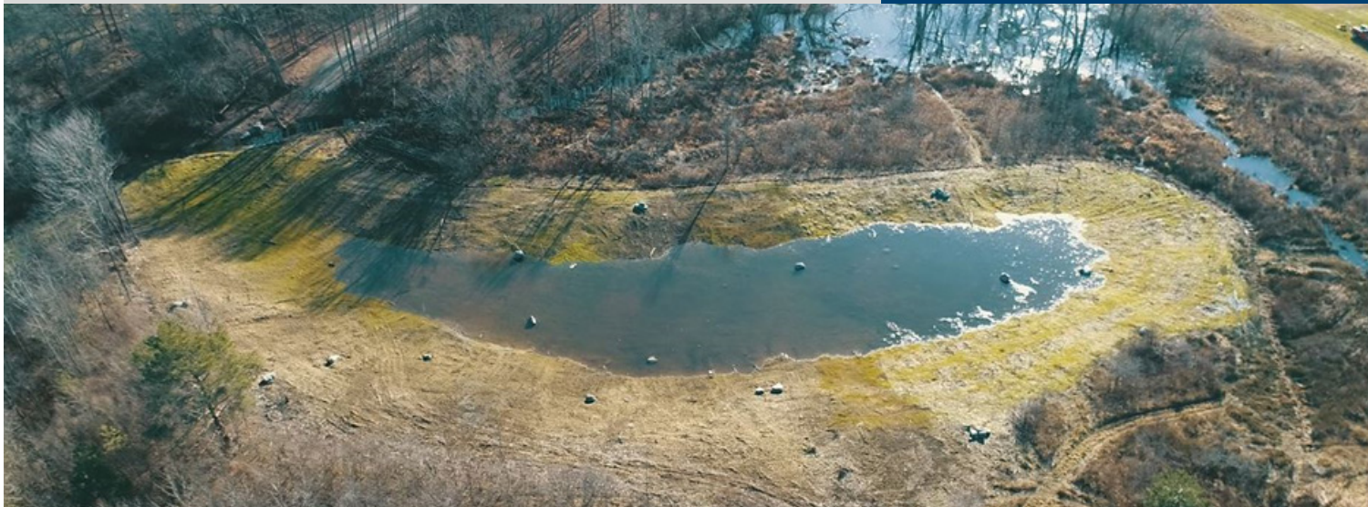
Wetland installed on a farm in the Skaneateles Lake watershed in Onondaga County. The project involved the creation of a 1-acre constructed wetland with an extensive floodplain capturing 2 million gallons during high flow events.
