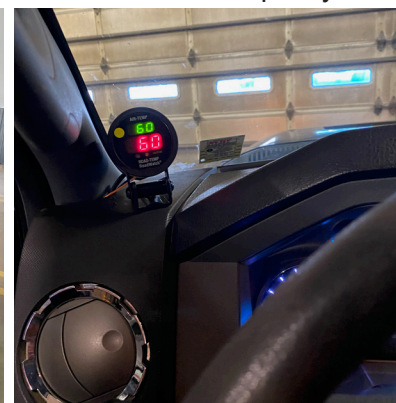
Left: Plow with adaptive blade retrofit to help remove ice from the road, using less salt. Right: Road temperature sensor to better gauge when to apply salt reducing the amount applied.
