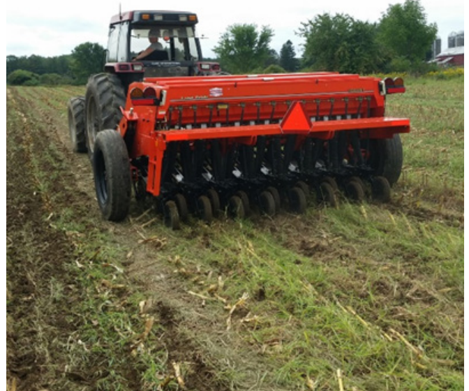
A no-till drill is used in Erie County to plant cover crops in the existing post-harvest crop residue.
