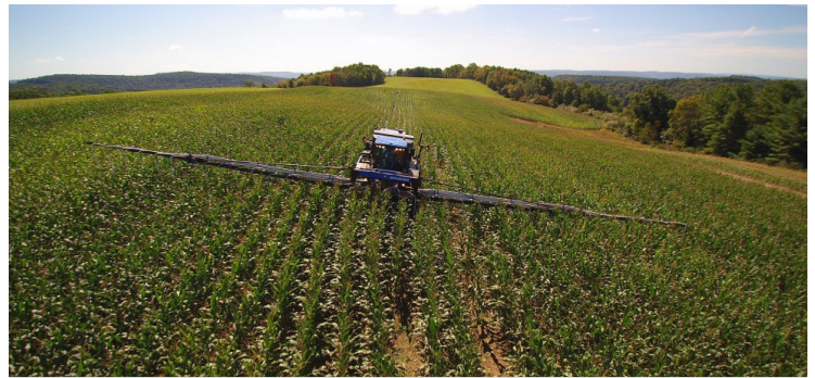
Schuyler County SWCD's Hi-boy interseeder funded through the SWCC's Climate Resilient Farming program is used to aid farmers in planting cover crops directly within an existing crop to improve soil health through reduced erosion, increased soil organic matter, and improved water retention.
